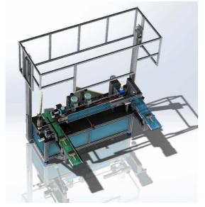
Straps transport system with speed regulation through inverter. Trimmers with blades .One trim head is fix and the other one is tracking system with brushless motor.
