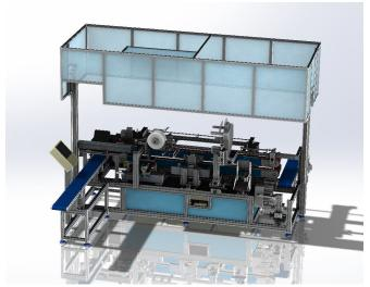
Brand new model that allows to obtain a packaging with coextruded film and with a hot melt glue diffuser, equipped of a mechanical pump with inverter that ensures a more accurate supply of the amount of glue.
