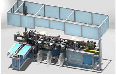
Head assembly with belt tran sport with touch screen for control and setup. Mechanical movements on skates and recirculating ball screws and management with 16 servomotors.
