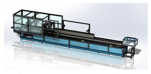
Machine for gluing and assembling the brush handle. It is equipped of three straps operated by brushless motors for the head transportation. Loading system with servomotor and brush alignment system. Glue dosing with translation system management in order to allow the uniformity of distribution Loading manipulator semi-automatic or automatic (IVM AM10).
